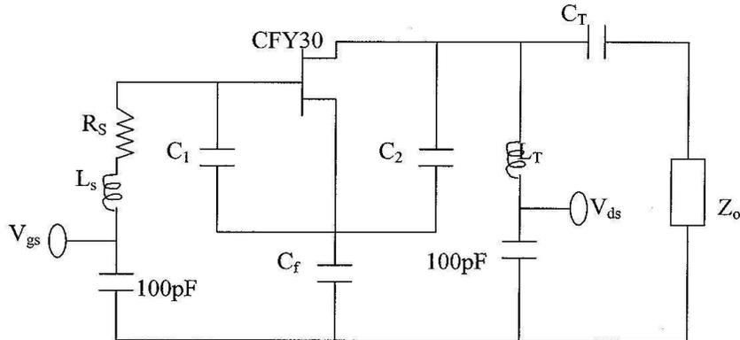
Figure 9 Schematic diagram of the oscillator operating at 950 MHz as published in [1].
