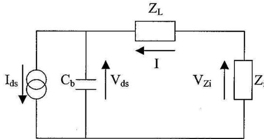
Figure 8 A circuit model of the oscillator.
