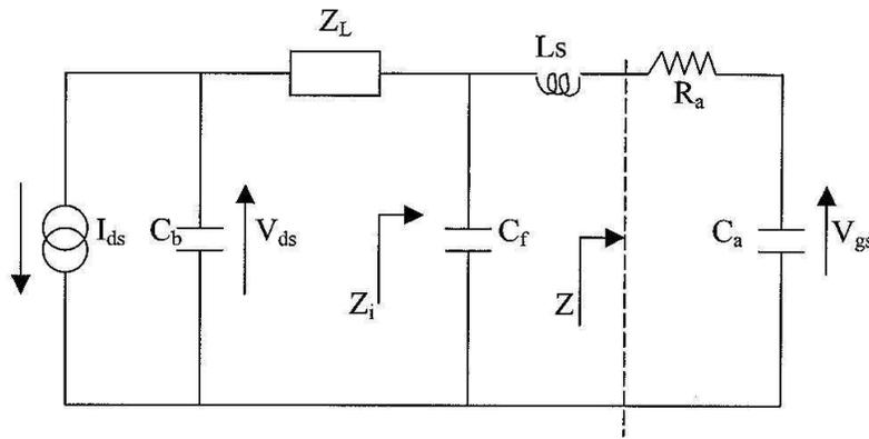
Figure 7 A simplified open loop model of the oscillator.
