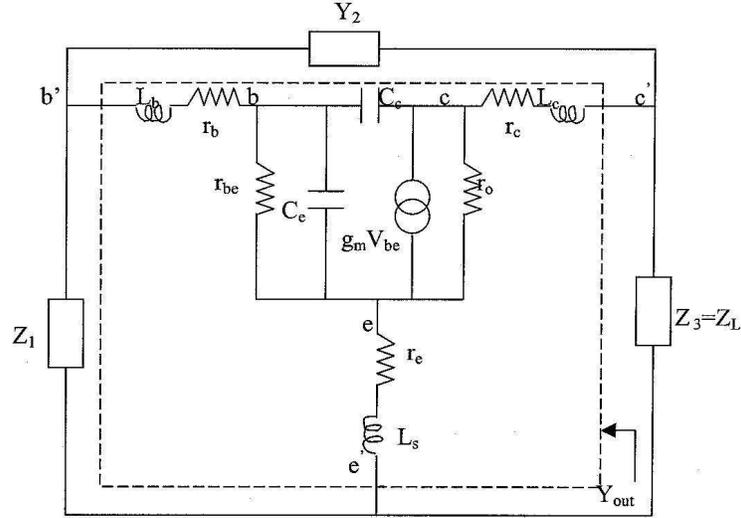
Figure 4 A parallel feedback topology of an oscillator using a bipolar transistor.
