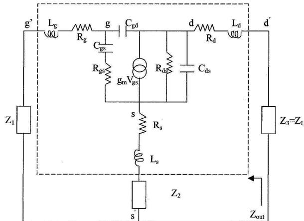
Figure 1 Series feedback topology for a MESFET oscillator.
