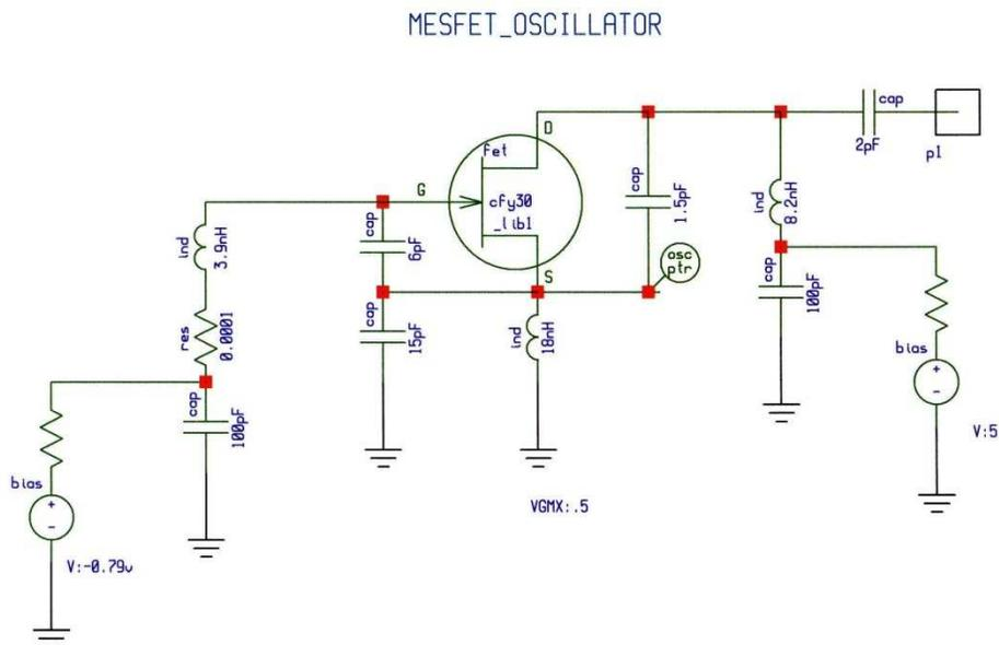
Figure 10 Schematic of the test oscillator based on [1].
