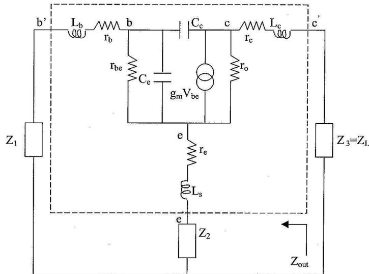
Figure 3 Series feedback topology of the oscillator using a bipolar transistor.
